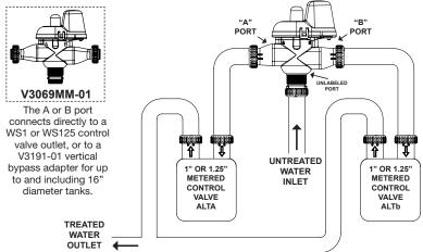
NOTE: When using the above setup, replace all V3003 meters with V3003-02 meters.
